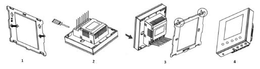
Step 1: Remove the steel frame from the device, and secure it onto the junction box with two screws.
